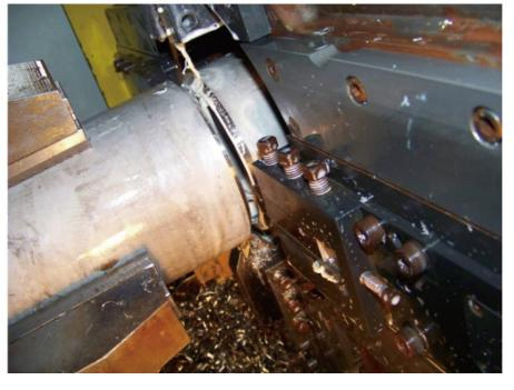
A high-quality and highly efficient integrated cutting and beveling process for small and medium-diameter thin-walled (≤25.4mm) pipes. This process is equivalent in efficiency to 10 sets of band saws and lathes combined. It takes only 2 to 3 minutes for cutting and beveling (two bevels) a 159 × 20 carbon steel pipe. One worker can replace ten workers. The savings in space occupation, labor cost, and electricity cost will recover the investment.
